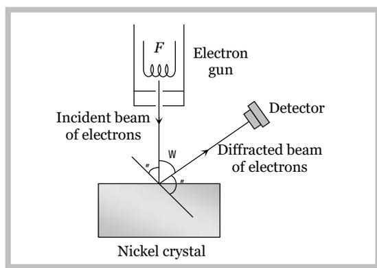
The diffracted beam of electrons is received by the detector which can be positioned at any angle by rotating it about the point of incidence. The energy of the incident beam of electrons can also be varied by changing the applied voltage to the electron gun.
