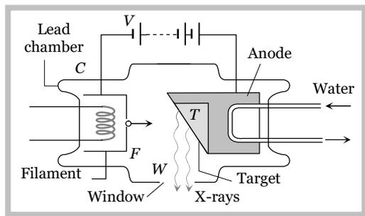
The filament is heated by passing the current through it. A high potential difference ( $\approx 10\text{ kV}$  to  $80\text{ kV}$ ) is applied between the target and cathode to accelerate the electrons which are emitted by filament. The stream of highly energetic electrons are focussed on the target.
