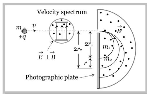
**Note** :  $\square$  Separation between two traces  $= d = 2r_2 - 2r_1 \Rightarrow d = \frac{2v(m_2 - m_1)}{qB'}$ .
