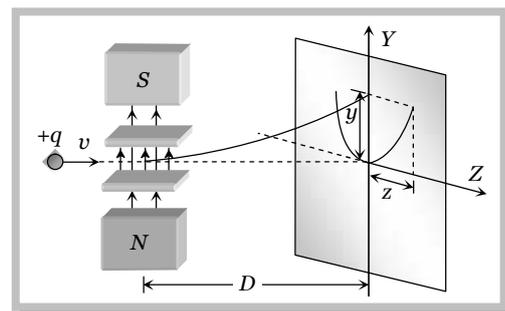
The positive ions are produced in the bulb at the left hand side. These ions are accelerated towards cathode. Some of the positive ions pass through the fine hole in the cathode. This fine ray of positive ions is subjected to electric field  $E$  and magnetic field  $B$  and then allowed to strike a fluorescent screen ( $\vec{E} \parallel \vec{B}$  but  $\vec{E}$  or  $\vec{B} \perp \vec{v}$ ).
